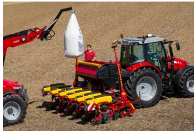
Tempo T can be equipped with a 1200 litre fertiliser hopper and disc fertiliser coulters.
