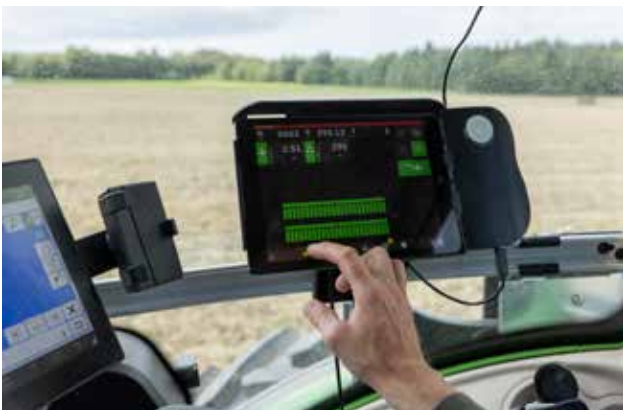
Seed Hawk 600-900C utilises the iPad based control system E-Control to monitor and control the seeding operation.
