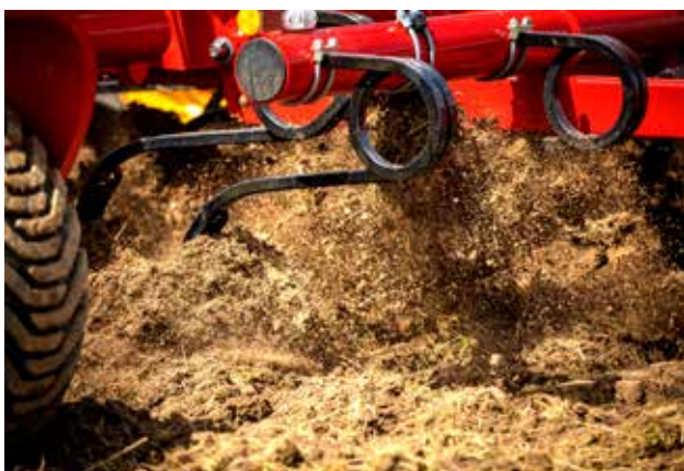
The vibrating Swift tines deliver an intensive mixing down to 20cm working depth.
