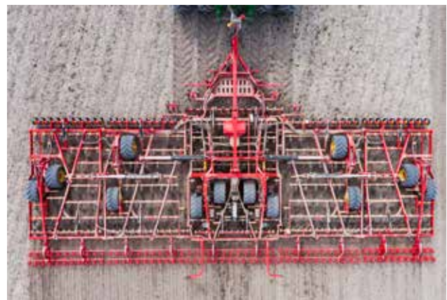
The wide OffSet bogie support wheels carries the NZ Extreme and maintains the working depth.
