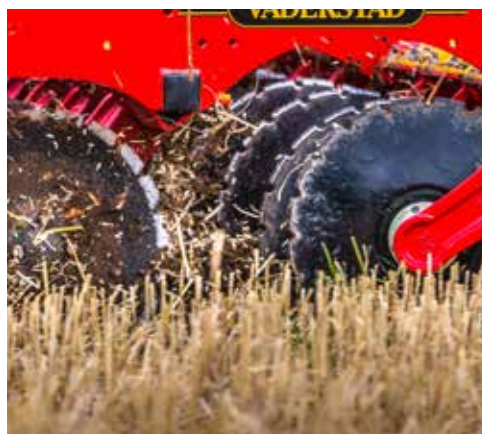
Two rows of high quality V-55 Swedish steel discs works down to 12cm working depth.
