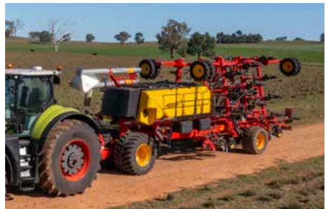
When transporting Seed Hawk 600-900C between fields, the machine is folded to fit within 3m transport width.
