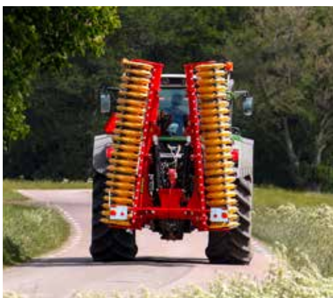
The transport width of the mounded Carrier XT is only 2.4m.
