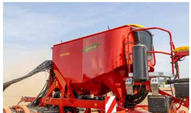
The seed-only model Spirit 600-900S holds 5000 litres.
