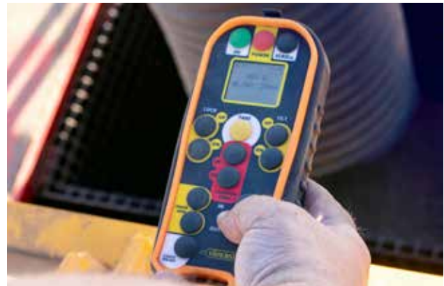
Fill System remote for PD 680-1350 Air Carts allows for wide functionality including belt speed controls while displaying real-time load cell values for each bin.
