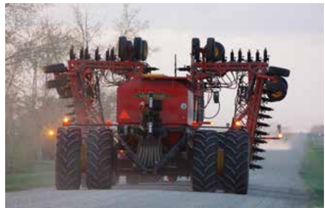
The toolbars are available in 5- or 7-section frames, enabling them to adapt to the contours of the land.
