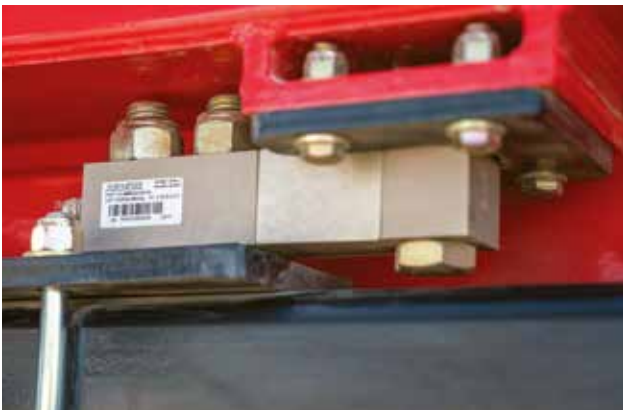
The modular tank design of Precision Delivery Air Carts feature individual compartment load cells.
