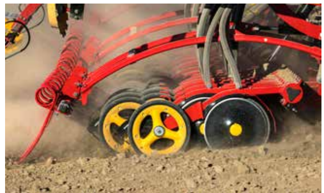
The seed coulters pressure, working intensity of the front tools or the pressure applied by the following harrow is easily adjusted from the cab on the move.
