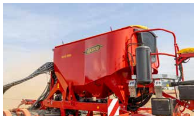
The seed-only model Spirit 600-900S holds 5000 litres.
