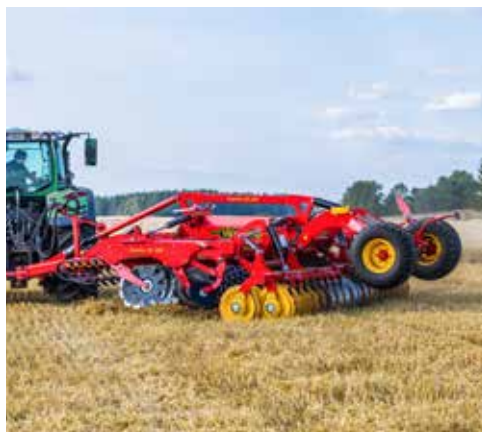
On headlands, the machine can be turned on either the packer or the wheels.
