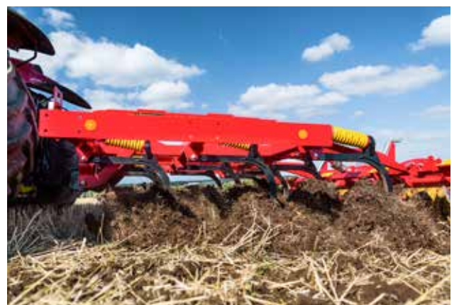
The Cultus and Cultus HD tines are able to work with high performance and depth consistency.
