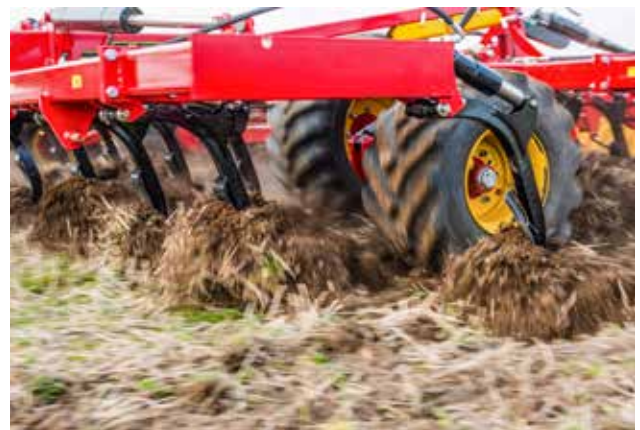
The powerful Opus tines are equipped with a stone release with up to 700kg release force. This ensures depth is maintained down to 40cm working depth.
