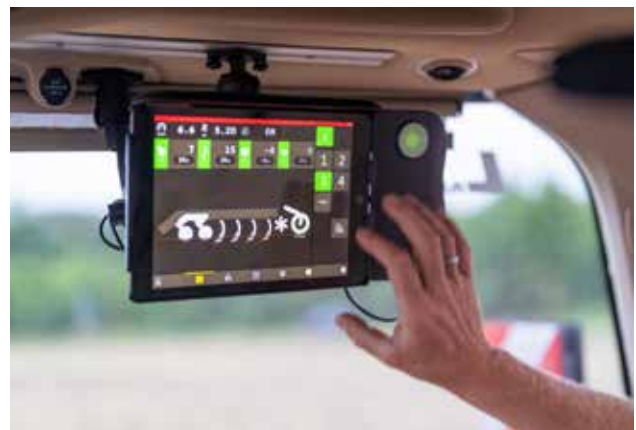
Equipping TopDown with the iPad-based E-Control system, enables full control as well as prescription map tillage.
