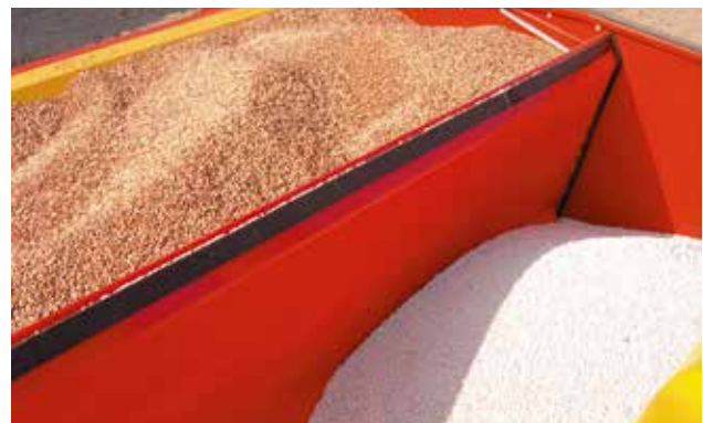
Rapid 300-400C/S has a high capacity hopper. On the combi models, the volume between seed and fertilizer is easily altered.
